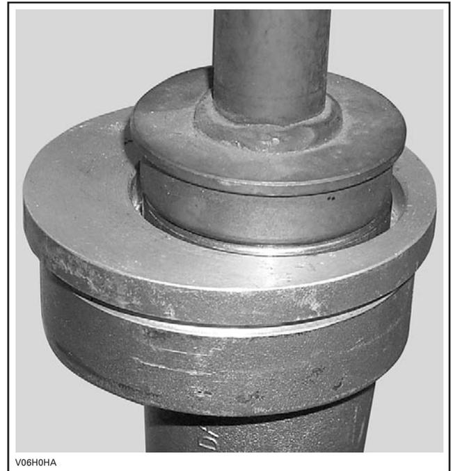
The seal must press into a dry bore. Use brake cleaner to make sure the bore is free of grease where the seal goes.
